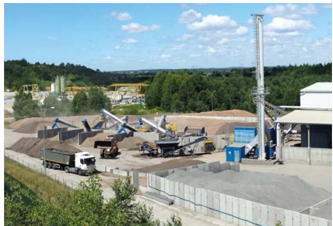
A pilot plant in Sowlany, Poland, produces 40,000 metric tons of lightweight aggregate annually.
